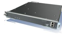
Figure 12: Cisco Wireless Services Module 2.
